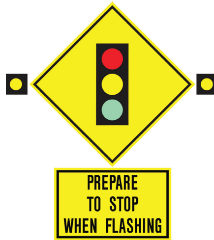
Figure 18 – Active Advance Warning Beacon
